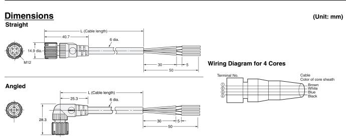
Note: The overmolding on the Standard Cable (XS5F-D42 -- 80-A) and the Oil-resistant Polyurethane Cable (XS5F-D42 -- 80-P) is black, and the overmolding on the Vibration-proof Robot Cable (XS5F-D42□-□80-F) is gray.
